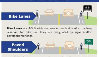
**Paved Shoulders** are sections along the sides of a roadway that are 4 ft or wider. They are open for all road users, including bikes and stopped motor vehicles
